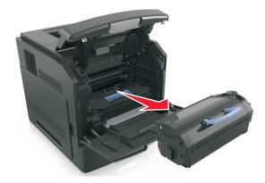
**3** Pull the imaging unit out of the printer using the handle.
